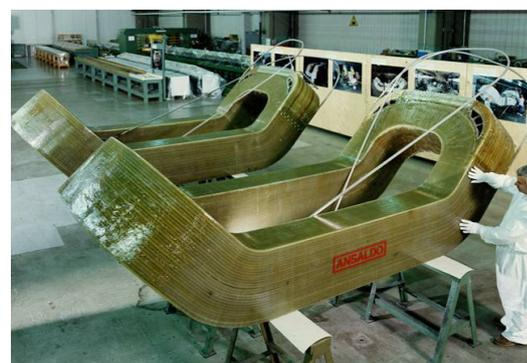
**Dipole coils after VPI impregnation**
